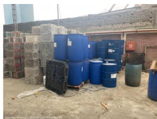
Chemicals are stored without secondary containment.jpeg
